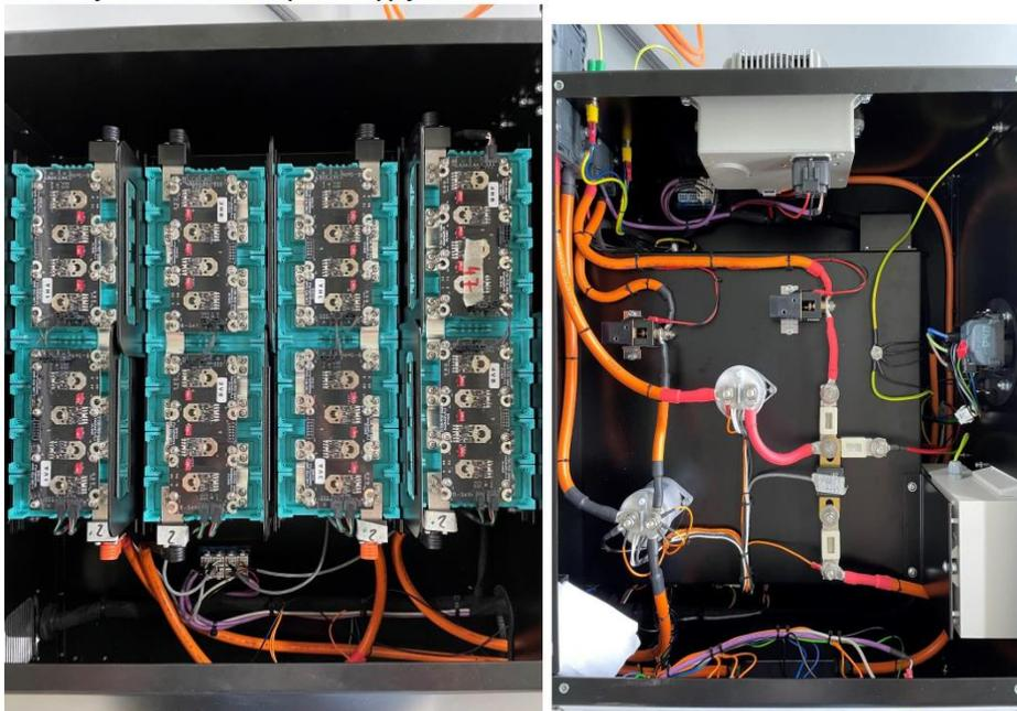
Functional model of e-drives and HV systems in motor vehicles
